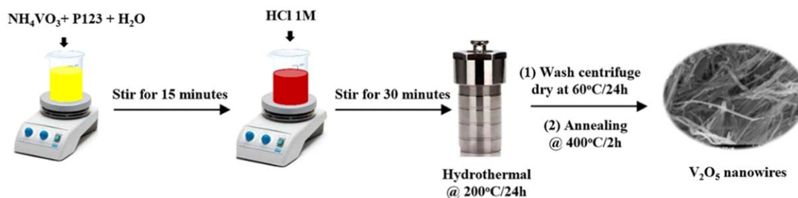
Figure 1. Schematic of hydrothermal synthesis of V_2O_5 nanowires.
